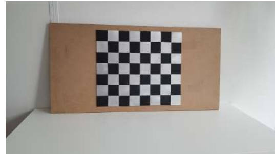
Figure 7: Chessboard used for calibration.
