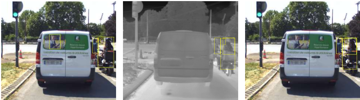
Figure 16: Difficult day example due to liveness detection difficulty. Left: results using only the visible modality. Right: results using our gated fusion method.
