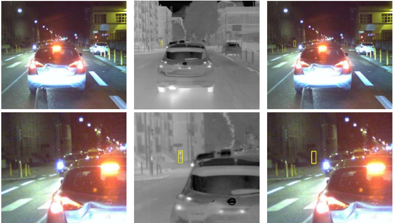
Figure 18: Difficult night example due to poor illumination. Top row: full image. Bottom row: zoomed on the region of interest. Left: results using only the visible modality. Right: results using our gated fusion method.
