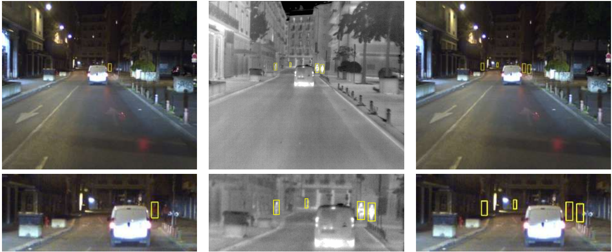
Figure 17: Difficult night example due to long distance from camera. Top row: full image. Bottom row: zoomed on the region of interest. Left: results using only the visible modality. Right: results using our gated fusion method.
